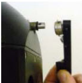
Figure 2.6: Remove Wiper Arm from wiper shaft
