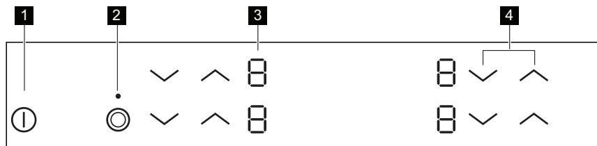
Use the sensor fields to operate the appliance. The displays, indicators and sounds tell which functions operate.
