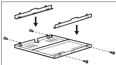
If you use a protection box (an additional accessory 1), the protective floor directly below the appliance is not necessary. You can not use the protection box if you install the appliance above an oven.
